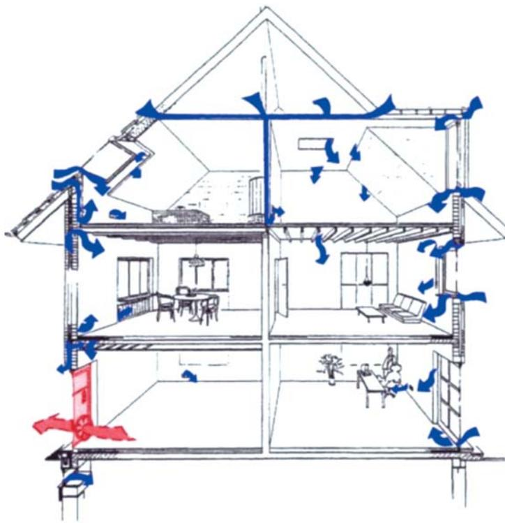
Figura 3. Test BlowerDoor.
